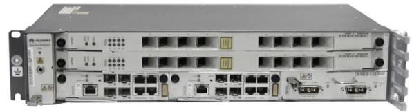
The MA5608T Mini OLT is designed to address Fiber to the premise (FTTP) or deep fiber deployment scenarios where a large OLT chassis may not be the best fit for a variety of reasons. Huawei's mini OLT MA5608T is designed to be the perfect complement to the other MA5600 series larger OLTs and offers the same carrier grade features and performance.
